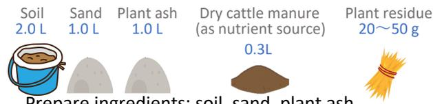
Prepare ingredients: soil, sand, plant ash, dry cattle manure, and plant residue. These are required to make one block (5kg).
